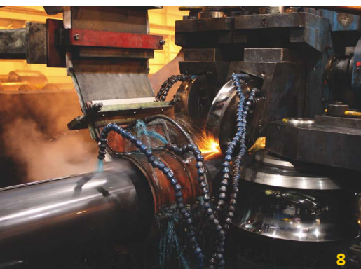
The edges are heat-forged together to form a complete circle.
