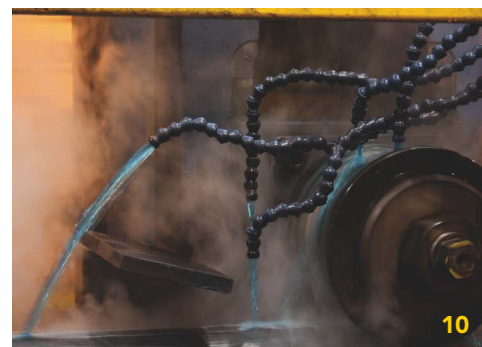
Steel is lubricated throughout the production line.
